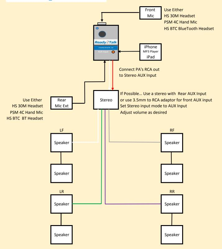
**Note:** If using 4 Ohm speakers connect pairs in SERIES If using 8 Ohm speakers connect pairs in PARALLEL
